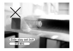
3. Insert the side stay straight, while keeping the upper and the lower staves horizontal. If you insert the side stay forcibly in an oblique state, it may cause damage to the side stay holder, the protective sheet or the stave.
