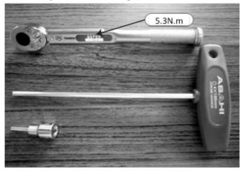
**Note:** Use a T – wrench for loosening the bolts, but avoid using the torque wrench except for assembling the side stay.
