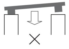
4. Insert accurately up to close contact so that no gap may be produced among the stave, the packing and the side stay.
